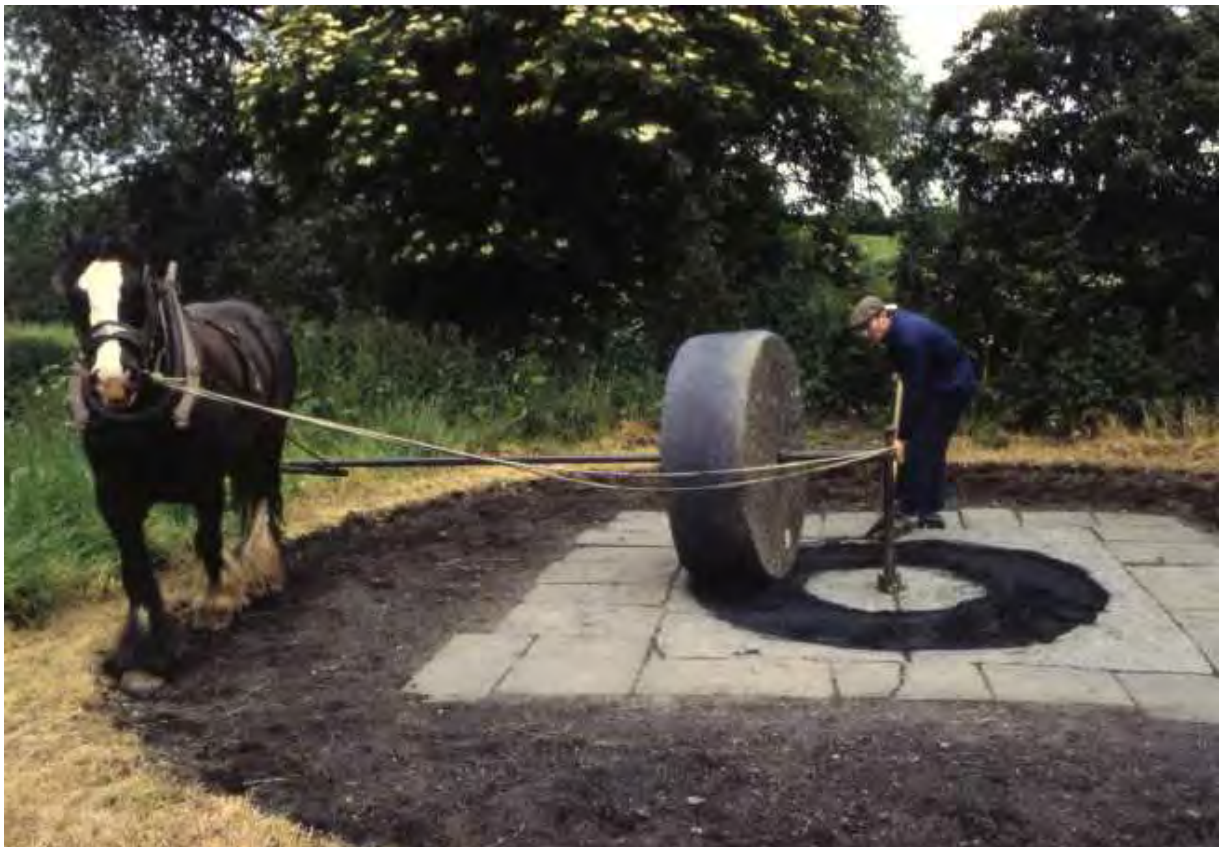
Culm crusher in operation, near Muine Bheag (Bagenalstown), Co. Carlow (Michael Conry)
